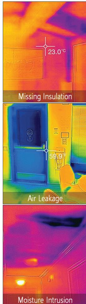
Figure 1: Common energy efficiency issues visible to a thermal camera.
