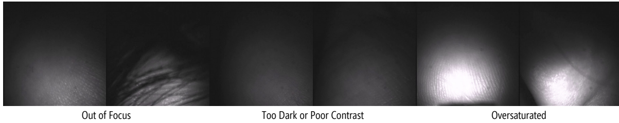
Fig. 4. Approximately 5% of the images we collected had poor focus, contrast, or illumination, preventing robust feature extraction. We adjusted the camera and LED to mitigate these issues for TouchCam Realtime.
