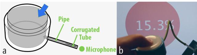
**Figure 6. The force sensor: (a) pressing the soft pad generates an air flow; (b) detecting different pressure force.**
