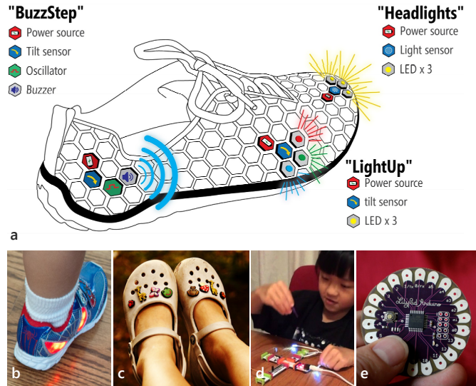
Figure 1: MakerShoe is an e-textile construction kit aimed at engaging young children (K-4) in wearable design. (a) Using only a few modules, this MakerShoe buzzes and lights up during movement and turns on ‘headlights’ when it’s dark. The bottom rows highlights a few inspirations including: (b) traditional light-up shoes, which are fanciful, fun, and responsive but not modifiable; (c) self-expression through fashion personalization (e.g., Crocs Jibbitz shoe charms); (d) littleBits electronic construction kit [1]; (e) and the LilyPad e-textile Arduino [3].
