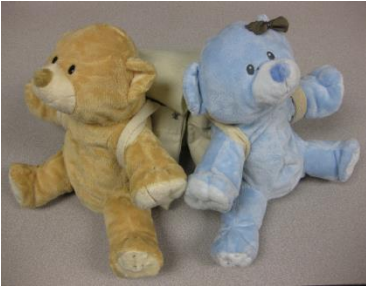
Figure 1. The Bear-With-Me prototype system consists of two bears that can sense and receive physical hugs and other forms of tangible expression in real-time over geographically distributed areas.
