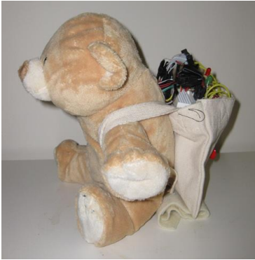
Figure 2. Profile view of Bear-With-Me bear. Each bear wears a custom fabric backpack that hides the Arduino microcontroller, WiFi shield, and other electronics.
