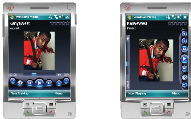
Figure 8. The left design is a typical music player, with targets near the screen bottom in “open space.” The right design has targets along the left and right screen edges, where elevated physical bezels improve accuracy when used in conjunction with the lift-off selection technique. Although round, the right-side targets would be made responsive all the way to the screen edge.
